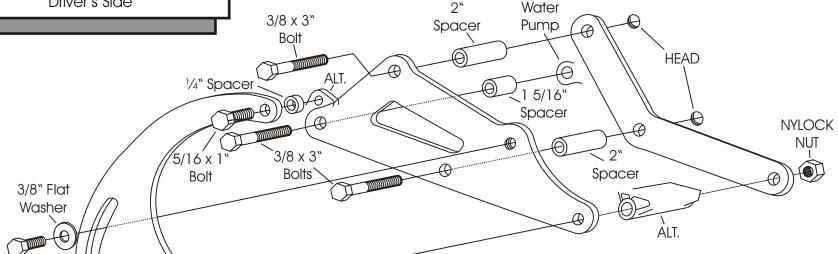
We use a belt length of  $55\frac{1}{2}$  -  $56\frac{1}{2}$  " with this mount on installations in our shop. However; this can vary with the diameter of your pulleys.
