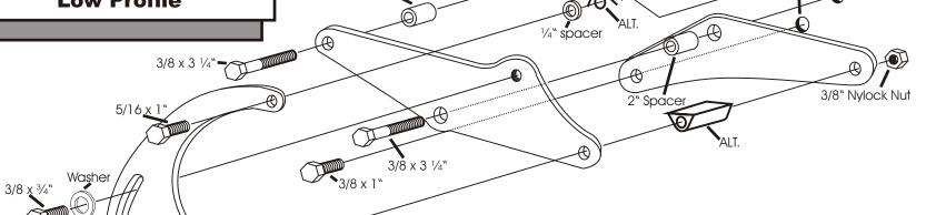
This bracket was designed to be used with Chevrolet double groove crank and water pump pulleys. The current G.M. part Numbers are 3744043 for the crank and 3995642 for the water pump.
