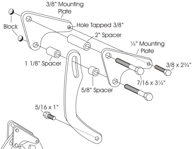
(We use a belt length of  $44\frac{1}{2}$  to  $45\frac{1}{2}$ " with this mount on installations in our shop. However; this can vary with the diameter of your pulleys.)
