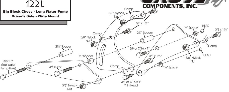
NOTE: Some heads have 3/8" bolt holes and some have 7/16". This kit includes both sizes of bolts for these holes.
