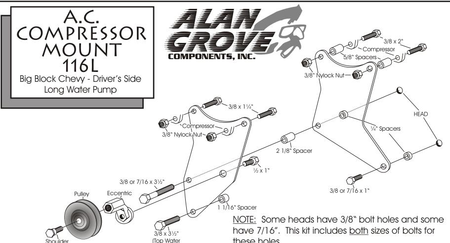
(We use a belt length of 57-58" with this mount on installations in our shop. This was determined using GM Part #14025185 crank pulley and Gm Part #14023155 water pump pulley.)
