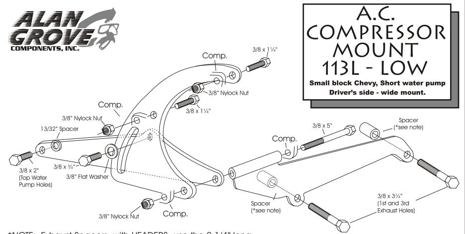
\*NOTE: Exhaust Spacers- with HEADERS- use the 2 1/4" long x 5/8" O. D. Spacers. With RAMS HORN MANIFOLDS use the 1/4" long x 3/4" O. D. Spacer at rear hole of bracket and a 1 1/16" long x 3/4" O. D. Spacer at front hole of bracket. With the later DROP-TYPE manifolds use the 1 1/16" long x 3/4" O. D. spacers at both bracket holes. As with any mount system, assemble all of the brackets to engine BEFORE TIGHTENING THE BOLTS.
