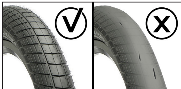
Recognising a worn tyre
