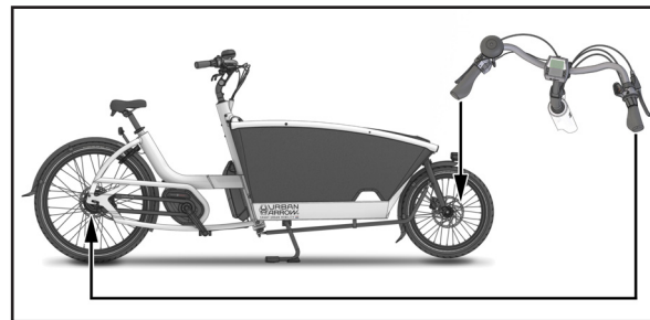
Brakes operated by respective levers
