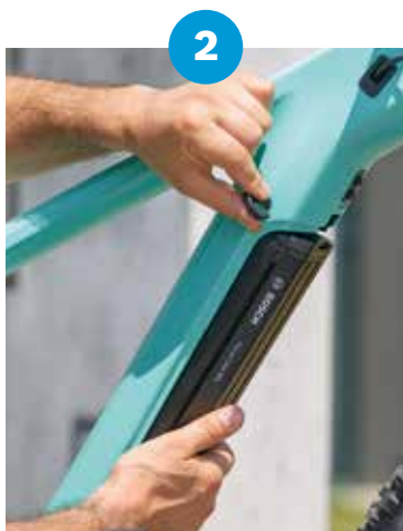
The battery is unlocked using a key and then falls into the restraint support.
