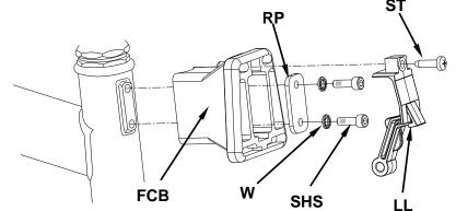
The screw 'ST' must be fully screwed home: If the latch is not properly locked in place, it will be ineffective and luggage may fall off, which is dangerous.
