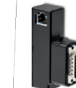
Audiolink-Converter (Art. No. 71600.080) Adapter for Loewe TV devices SL2xx / SL3xx / SL4xx with previous sound systems (digital audiolink to analogue audiolink / 26 pin D type connector). Can be used in combination with adapter (Art. No. 89954.101) to connect Loewe TVs to old Loewe subwoofers without audio link connection and 3rd party audio systems.
