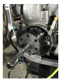
Figure 3 Flywheel torqueing
