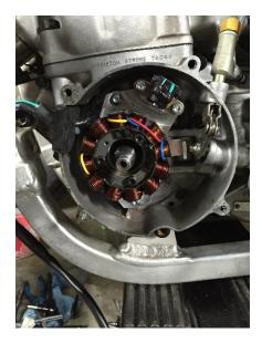
Figure 2 Stator installation
