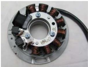
Insert the new base plate with the stator in the place of your old stator and fasten the plate with the two provided M5 screws (Please don't use other screws, as they may be too high and could scratch at the rotor).
