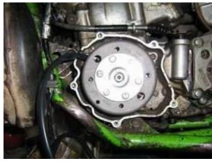
In this position fasten the rotor carefully with the screw provided.
