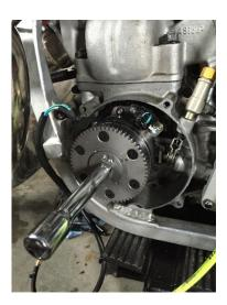
Figure 1 Flywheel torqueing
