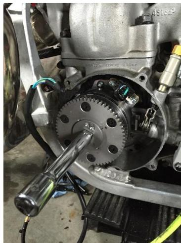
*Figure 3 Flywheel torquing*
