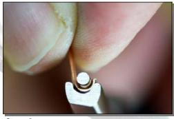
Step 2 Squeeze the jaws closed to start the U-bend in the wire.
