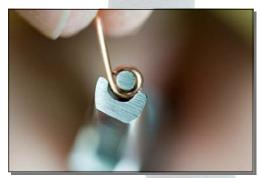
**Step 4**Rotate the pliers to bend the wire back on itself to make a complete loop.
