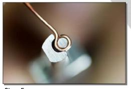
Step 5 When the loop is closed, rotate the pliers back slightly allowing the concave jaw to bend the excess wire away from the loop,
