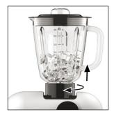
Unplug the appliance and wait until the blades have stopped rotating. Slightly turn the blender to the left to unlock, then pull it up to release from the top attachment port.
