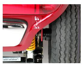
brakes, your scooter can still be freewheeled by lifting the front of the unit and pulling, using the base of the tiller as a secure handhold.
