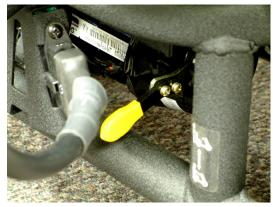
To switch to "Freewheel" mode, locate levers situated at the front of both motors and behind each front wheel and move both levers outward. Advice indicators are shown at this location. To re-engage motors/brakes, move both levers toward the center.
