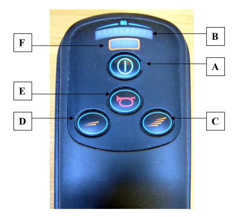
Your Powerchair is fitted with the latest up to date electronic controls. The "joystick control box" Photo # 4 is normally fitted to the right side of the chair. Switch on your Powerchair with the ON/OFF button (A). When the chair is turned on the Battery Indicator lamp (B) lights up. This also can be used as a fault guide. The chair is ready for use if the green battery level indicator bars are illuminated (B). The range of the Powerchair is relative to the number of bars lit.
