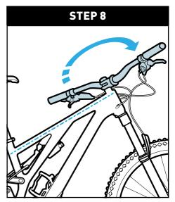
Brace the wheel between your knees and rotate the handlebar into alignment.
