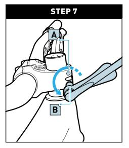
Using the torque wrench and corresponding hex bit, loosen (counter-clockwise) the two bolts (A-B) on rear of the stem until the stem is loose enough to turn.
