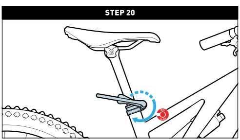
Using the torque wrench and corresponding hex bit, torque the seatpost collar bolt to the specified torque setting found on the seatpost collar and/or in the user manual (where applicable).
