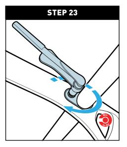
Once the seatpost height is set, use a torque wrench and corresponding hex bit to torque the wedge bolt to specification.
