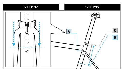
The seatpost must be inserted into the frame deep enough so the minimum insertion/maximum extension (min/max) mark, where applicable, on the seatpost is not visible **(A)**.
