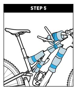
Remove the zip ties or rags securing the handlebar to the top tube.
