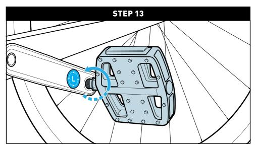
Insert the "L" pedal into the left (non-drive side) crank arm.
