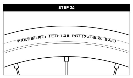
Pump the tyres up to your desired pressure. Refer to the tyre's sidewall for the pressure range. Check your wheel manual or decal on the rim itself to see if your wheels have a maximum pressure limit. Do not exceed it.
