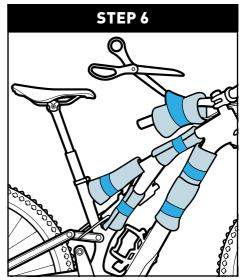
Remove the zip ties or rags and protective packaging from the rest of the frame.
