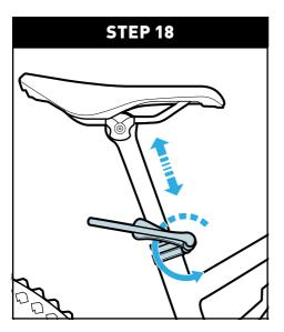
Using the torque wrench and corresponding hex key, loosen the seatpost collar bolt and set the saddle height to your desired position, then lightly tighten the seatpost collar bolt.
