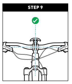
Align the handlebar with the center of the bicycle.
