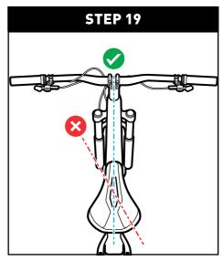
Align the saddle with the centerline of the bicycle.
