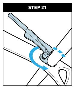
Using the wrench and corresponding hex bit, loosen the seatpost wedge bolt.
