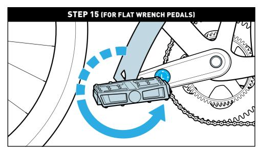
Using the flat wrench, tighten the pedal in place (counter-clockwise rotation). When at the correct tension, the tool leaves a noticeable impression in the palm of your hand.
