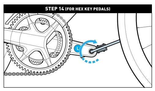
Using the corresponding hex key inserted from the inside of the crank arm, tighten the pedal in place (counter-clockwise rotation). When at the correct tension, the tool leaves a noticeable impression in the palm of your hand.
