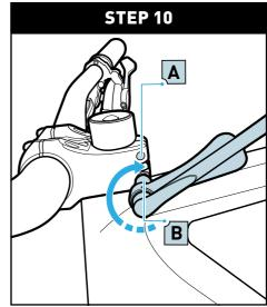
Using the torque wrench and corresponding hex bit, torque (clockwise) the two bolts (A-B) on rear of the stem to specification.
