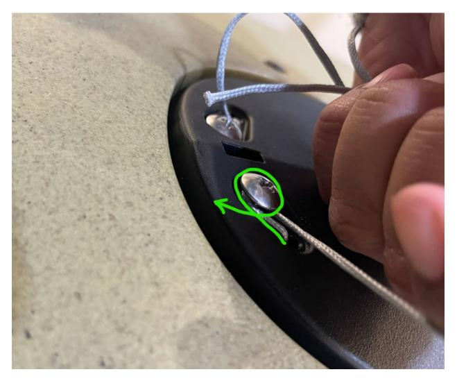
Finally, feed the line through the hole in the center of the drum.
