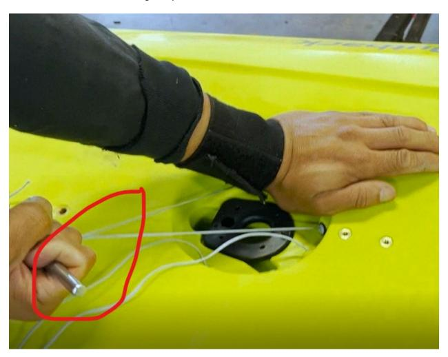
Tie the lines around a tool and tug firmly on the line. This will stretch the lines and remove the slack.
