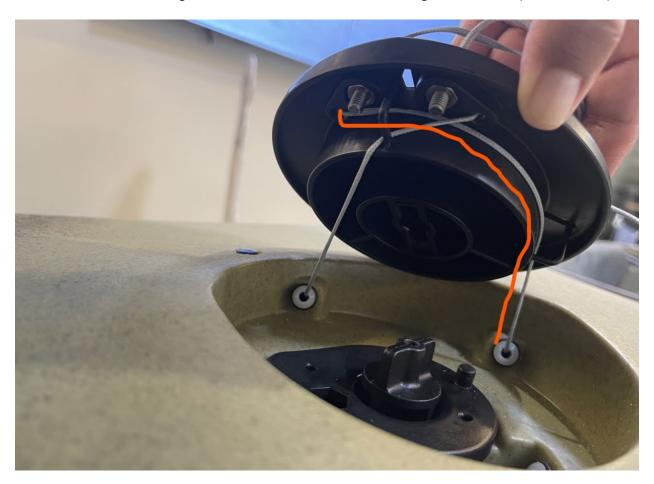
Weave the left line to the right of the drum and the left line to the right of the drum (as seen below).
