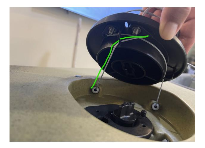
Once the lines are woven through the drum, screw the rudder drum into the rudder housing (the screw in the middle of the drum).
