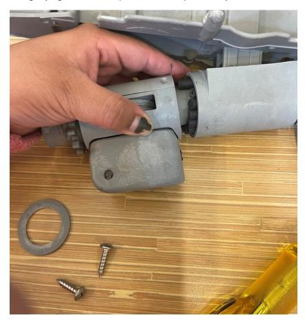
7. This is the result of #6. Some bearings may have fallen into the hole visible in the sprocket.
