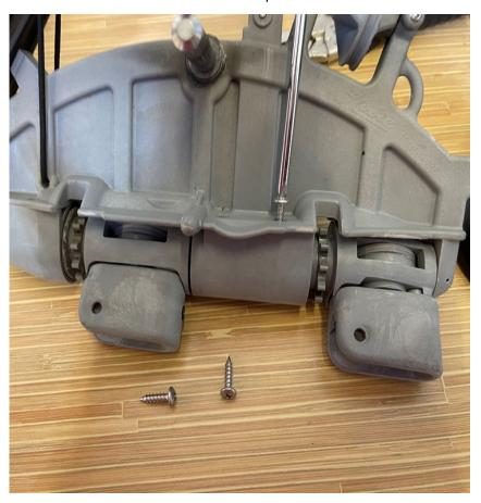
2. Give a light tug to the center sprocket to loosen it.
