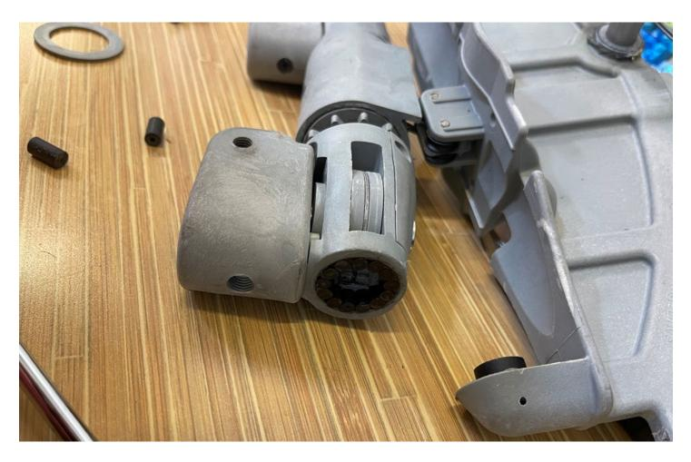
14. Pull on the spectra line to bring the center sprocket further up. Next, reinstall the smallest sprocket on its base. Then, push up to reinstall the center sprocket. You may need to pull on the line more.
