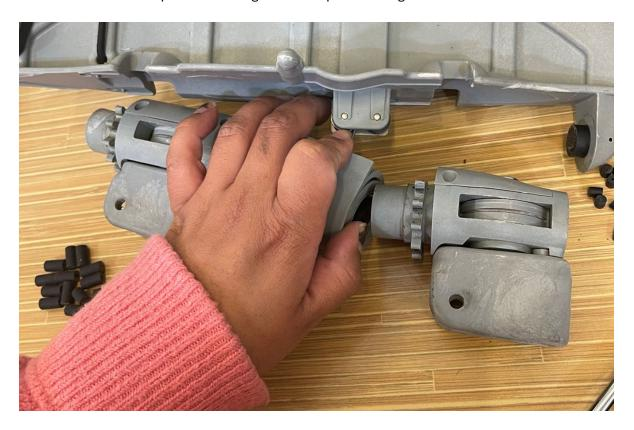
13. Add grease to the smallest sprocket and install the bearings.
