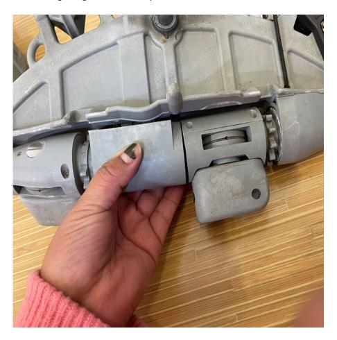
3. Remove the bottom screw on the sprocket.
