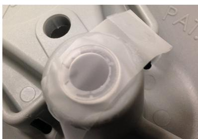
A piece of tape can be used to hold plastic bearing retainer in place during installation.
