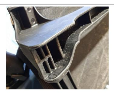
The seat risers are made to attach to the 4 points on the base of the chair. All you need to do is on each point, line the riser up with the edge and then drill a 3mm hole and screw the self-tapping screw in to hold it in place.
