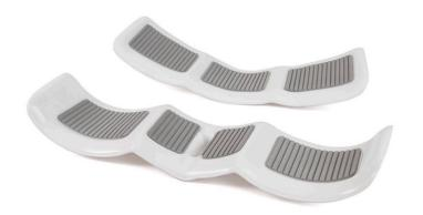
Before you install the cradles, note that there is a front and back direction to each cradle. Your 2019+ Hobie Outback is widest in the middle and tapers at both the bow and stern. The forward cradle is narrower at the front. The aft cradle is narrower at the back and the channel for the keel is slightly larger at the back.
