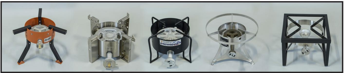
**BURNER TYPE** is also an important consideration. Cup style burners, such as the Adventures in Homebrewing (AIH) unit, are very inexpensive to manufacture, put out a reasonable amount of heat, but are very loud. Nozzle type burners were used in all but the AIH burner. They are quiet and efficient until you exceed a certain fuel/air flow where the flame lifts and becomes unstable. While you can continue to increase the power output, they do become louder and the efficiency drops.
