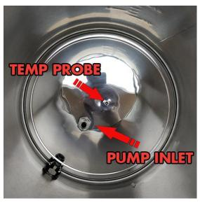
The photo to the right shows the placement of the probe. The probe placement has been designed like this as it prevents the element from overheating and scorching wort by taking the temperature of the wort closest to the element. This is why your strike temperature needs to accurate!
