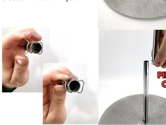
Now place use the extension tube and place this on top of the other stainless tube that you just attached to the bottom screen
