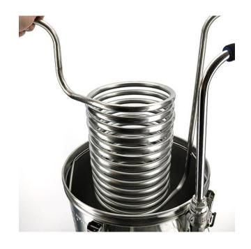
Compression fittings for the immersion chiller can be purchase separately if you want to use threaded connections for camlocks or garden hose fittings. (see picture below - part number KL02004). This will enable any ½" BSP threaded fitting to be attached.
