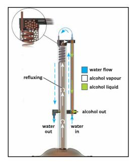
The saddles in the column provide a large surface area to maximise the contact between the liquid and vapour flows in the column, and accelerate the refluxing action.
