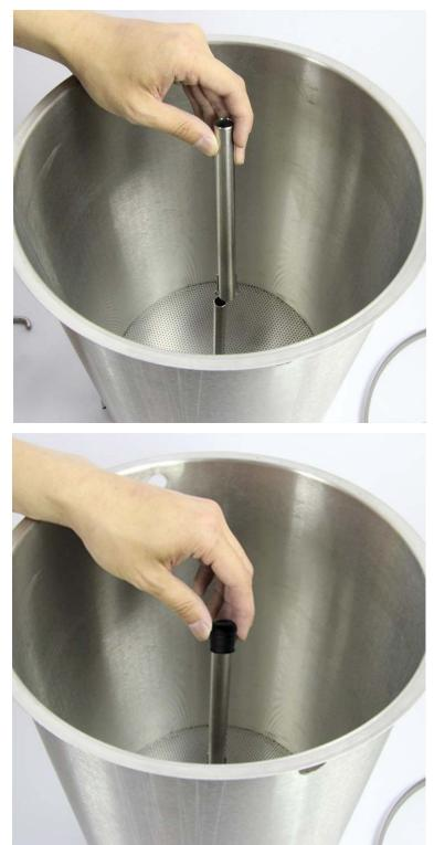
We recommend installing the malt pipe handle <u>before</u> you add your grain and malt pipe into to your RoboBrew.
