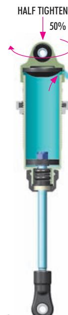
5 Gently place the shock cap assembly onto the filled shock body. Excess oil will spill from the shock. Screw the shock cap onto the body by only a few turns.
