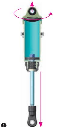
**1** Extend the shock shaft completely and remove the shock cap.
