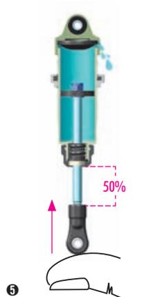
**5** Push the shock shaft 50% into the shock body. Excess oil will bleed through the hole in the shock cap.
