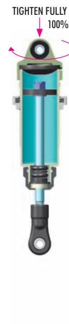
7 Keep the shock shaft pushed in the shock body and tighten the shock cap completely. The rebound will be at approximately 0%.
