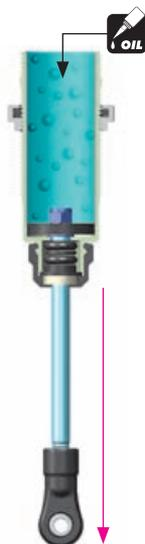
1 Extend the shock shaft completely. Fill the shock body with the shock oil. For the shocks use 800cSt oil.
