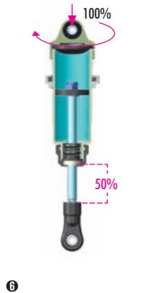
**6** Keep the shock shaft pushed 50% into the shock body and tighten the shock cap completely. The rebound will be at approximately 50%.
