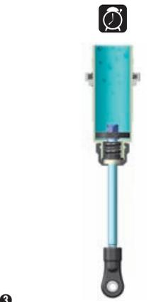
**4** Gently place the shock cap assembly onto the filled shock body. Keep the shock shaft extended 100% from the shock body and tighten the shock cap completely. The rebound will be at approximately 100%.
