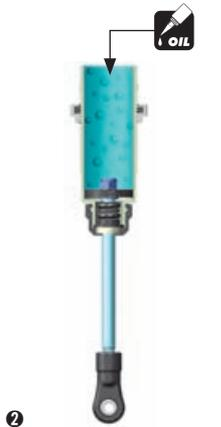
**2** Fill the shock body with shock oil up to the top. Make sure to use same viscosity shock oil as is in the shock.
