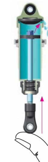
6 Gently push the shock shaft completely into the shock body. Excess oil will flow through the hole in the shock cap.
