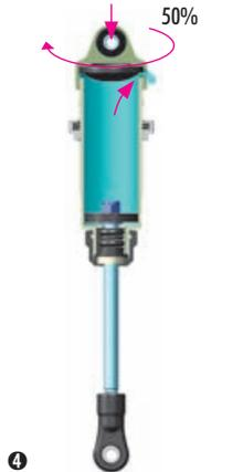
**4** Gently place the shock cap assembly onto the filled shock body. Excess oil will spill from the shock.
