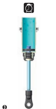
**3** Orient the filled shock vertically for several minutes with the shock shaft fully extended. The remaining air bubbles will release.
