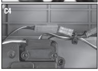
C5. Use the included zip tie (1) to secure the harness to the chassis (refer to Fig. 2 Chassis Wiring for more detail).
