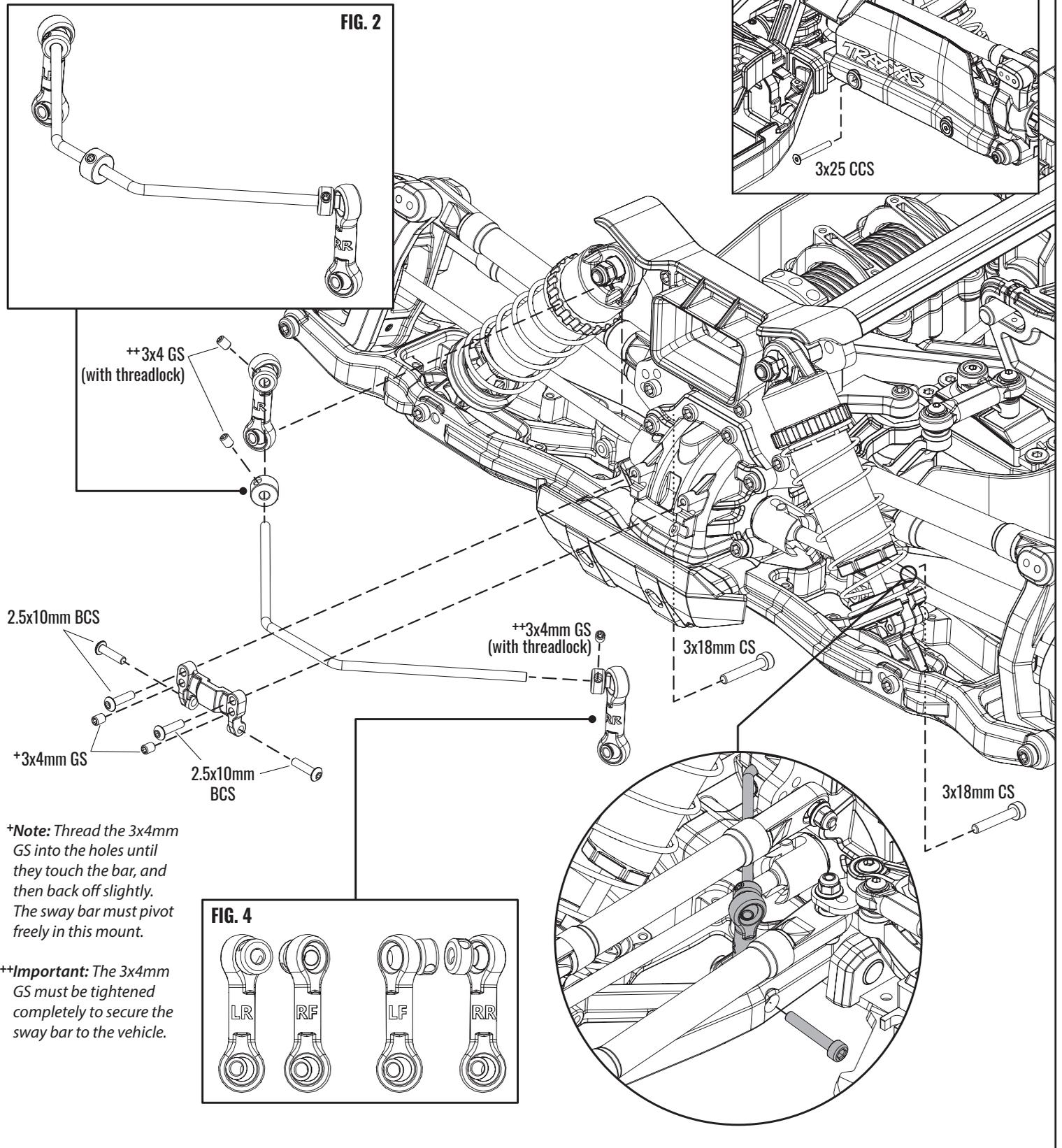
**\*Note:** Thread the 3x4mm GS into the holes until they touch the bar, and then back off slightly. The sway bar must pivot freely in this mount.
