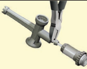
C. Remove/Install Rod End
