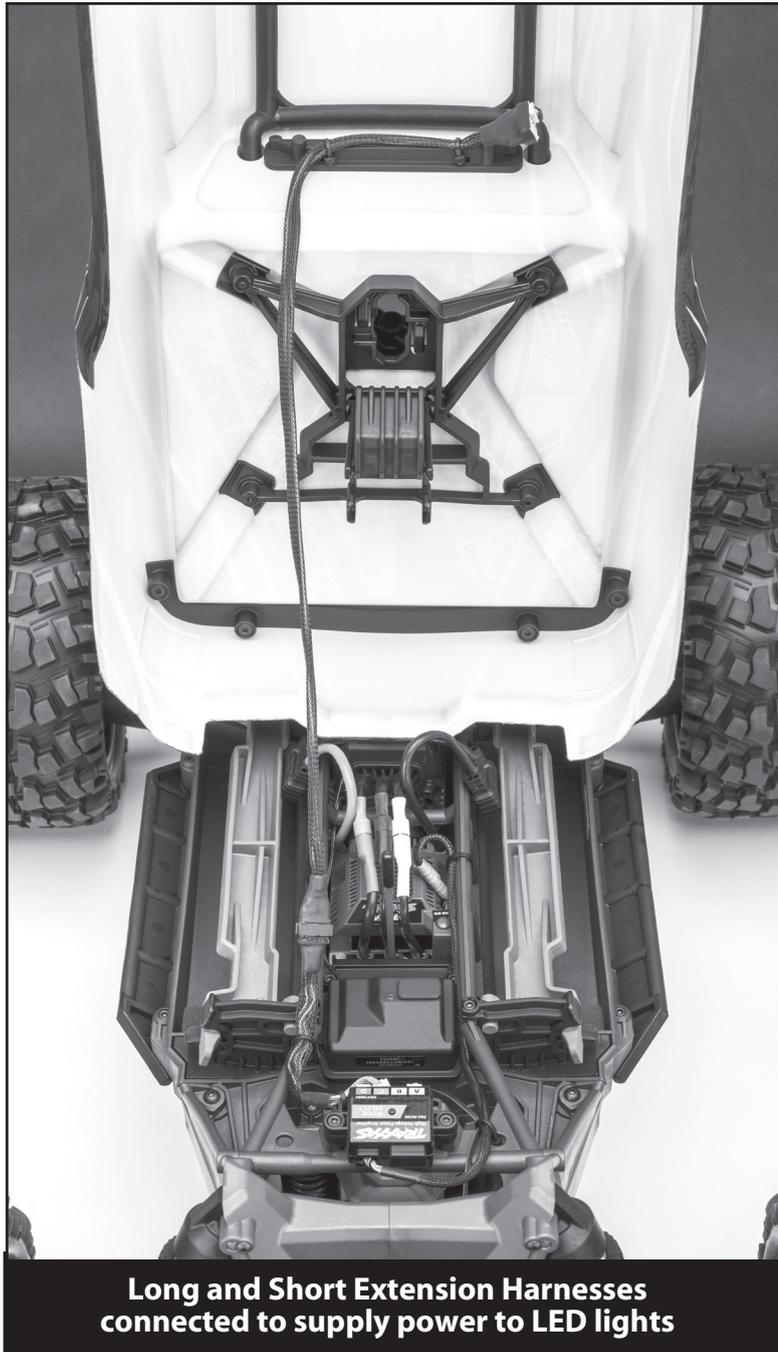
**Long and Short Extension Harnesses connected to supply power to LED lights**
