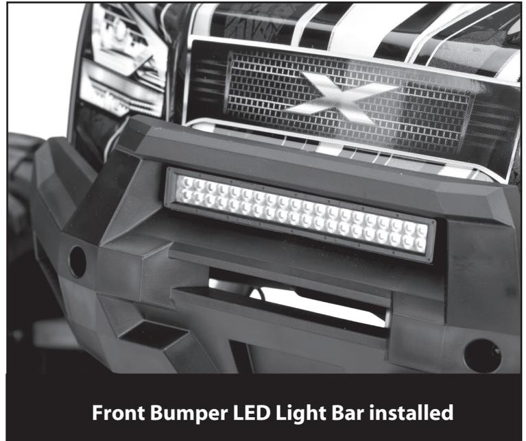
**Front Bumper LED Light Bar installed**
