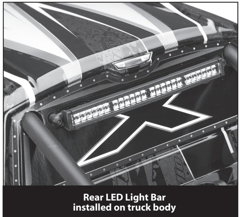
**Rear LED Light Bar installed on truck body**
